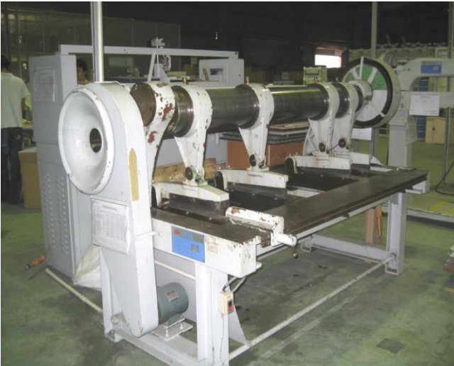
SLOTTER MACHINE (use for Plastic and Paper Box)
