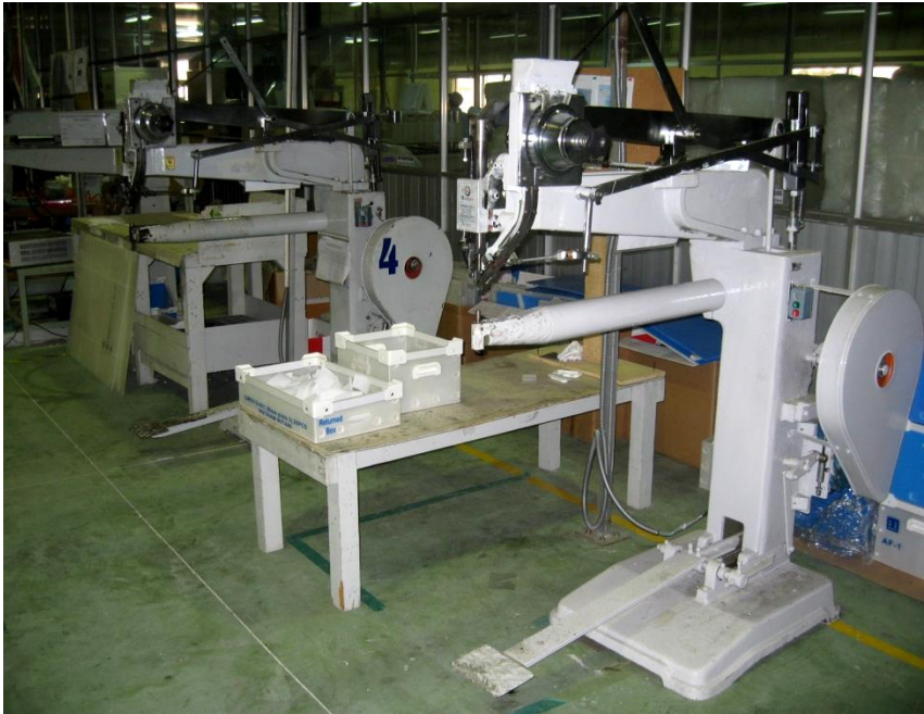
RIVETER MACHINE (use steel and plastic Rivet for Danpla Box)
